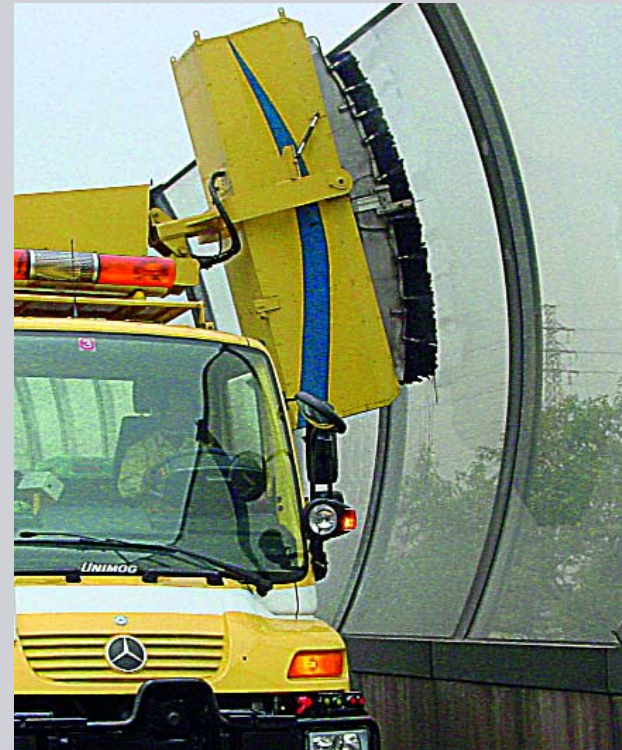
Pulling out all the stops - the Unimog U 400 with curved, rotating brush.
