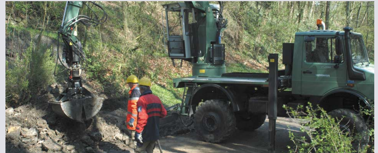
Unimog U 5000 with Ematec M 213 loader: an essential part of the bomb disposal unit.
